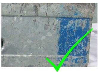
Colour markings for the distinction between the different element types of the same size must be visible. (Universal element, Frami anchoring element, 0.55m wide elements),
