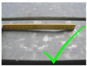
Allowed on one side of frames and cross profiles up to a length of 80mm.
