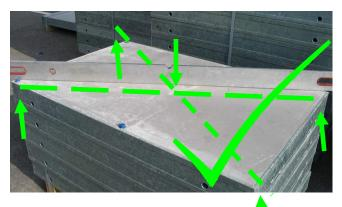
3 mm per element length allowed. At Frami 2,70/3,00m 5mm distortion allowed.
