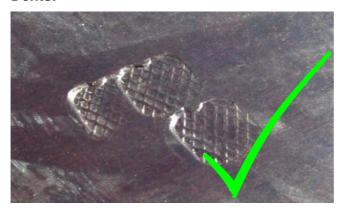
Up to a size of 2 patches D60 and a depth of maximum 1mm allowed.
