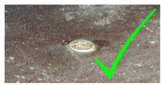
Must be complete and have tight seat. Beam holder, steel waling, lifting bracket and/or screwing plate. At fixing ledges 1 missing screw each 1,20m allowed.
