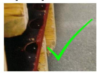
Continuous frayed spots of a maximum size of 30 x 3mm are allowed. Frayed spots of a size of 50 x 5mm up to 20mm in width are allowed selectively. But this may not lead to leakage at stacking. Parts that are sticking out must be grinded off and sealed by varnish.
