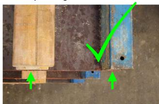
Plywood overlap up to 3mm allowed. The beam may overlap the panel up to 1mm.
