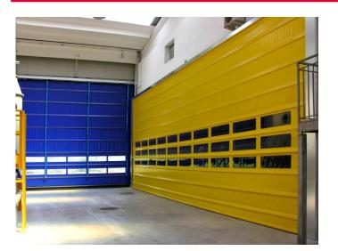
The High-speed folding door 650 is a fast folding door designed for large industrial passages with intensive use and resistant to high wind pressure. The maximum dimensions of the High-speed folding door 650 are 12.000 x 10.000 mm (wxh).
