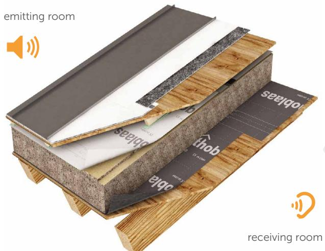
The effectiveness of TRASPIR METAL was demonstrated through an airborne soundproofing test and noise generated by heavy rain.
