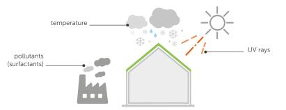
In order to maintain the properties of the product, it is important to choose it taking into account the conditions it will be exposed to throughout its life, from construction to operation, and to protect it as much as possible (the construction phase is a source of stress and accelerated ageing).
