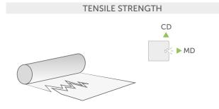
Force exercised both longitudinally and transversally, to determine the maximum load, expressed as N/50 mm.
