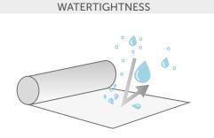
Ability of the product to temporarily prevent the passage of water during construction and in case of accidental breakage and dislocation of the roof covering.
