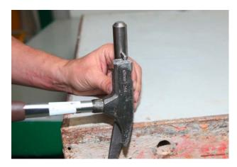
Insert new rivet and fix it by using a pneuamtic or electric rivet gun.
