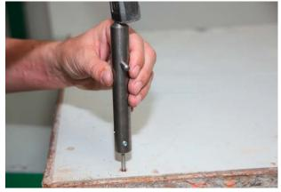
... then remove rivet by using a hammer.
