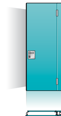
FT Fixed pass door The telescopic panel can be replaced by or used in conjunction with a fixed pass door. The pass door is full height and is fixed to one end of the existing building structure. The door is equipped with pressure seals at the top and bottom, which extend automatically during the closing action of the door.
