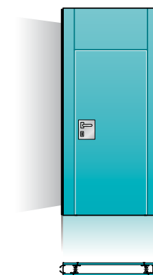
DT Pass door panel (single hinged) This fully moveable pass door is constructed with a high-quality welded steel frame. This solid construction makes any type of floor track or locking mechanism redundant. The door is equipped with a pressure seal at the bottom, which extends automatically during the closing action of the door. During sliding of the pass door panel, the door will be secured automatically.
