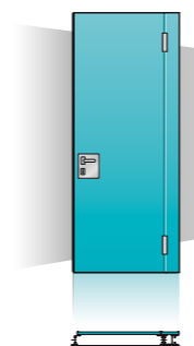
FT Fixed pass door The telescopic panel can be replaced by, or used in conjunction with, a fixed pass door. The pass door is full height and is fixed to one end of the existing building structure. The door is equipped with pressure seals at the top and bottom, which extend automatically during the closing action of the door.
