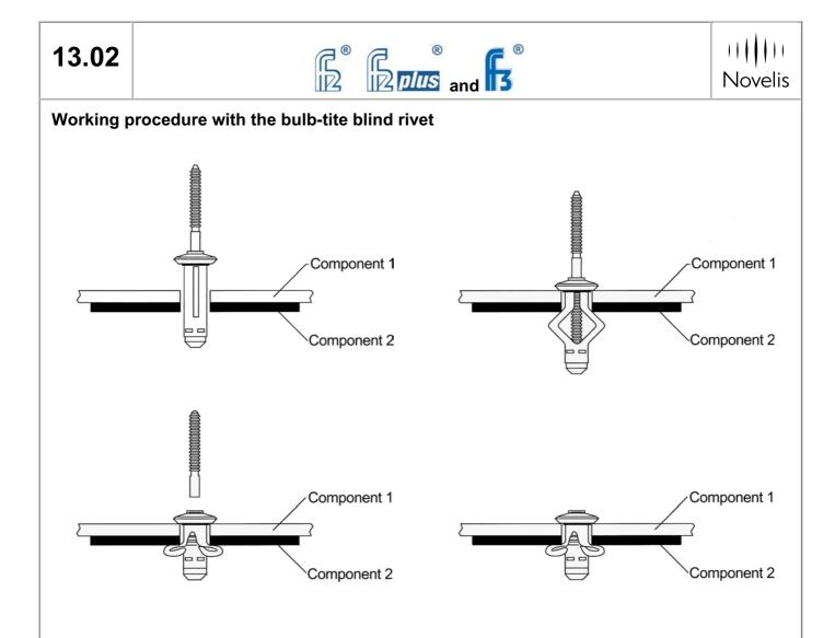
A special mouthpiece is required for the bulb-tite blind rivet.
