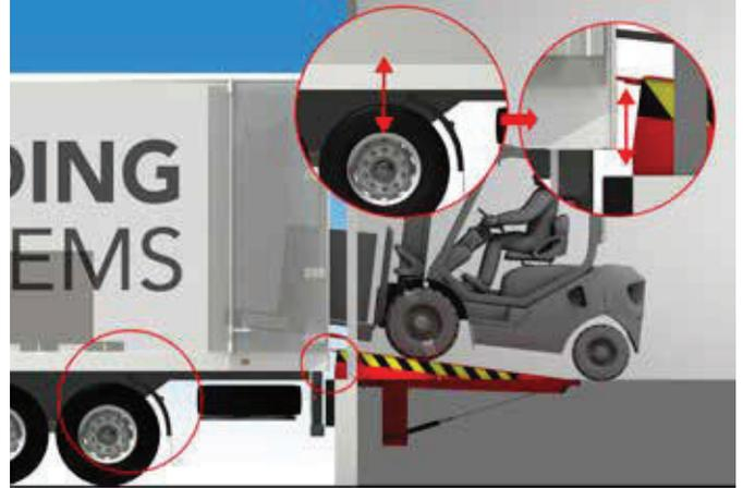
The Loading Systems dock levellers are also suited to load or unload so called end loads below warehouse level.
