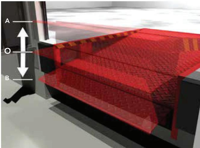
In compliance with EN 1398 it is not permitted to use dock levellers outside the permitted gradients of  $\pm 12.5\%$  (approx.  $\pm 7^\circ$ ).
