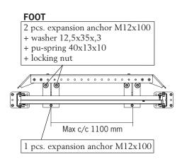
The frame protector fulfill the requirements according to SS-EN 15512, even during assembly without pu-spring. We recommend that the pu-springs are always installed, since it increases the frame protectors capacity against repeatedly collisions.
