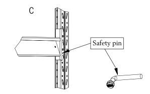
5. Raise the first section and fit two safety pins per horizontal beam
