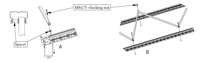
3. Place a spacer at free side of horizontal brace
